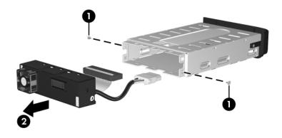
Removing the Hard Drive Carrier Rear Panel
